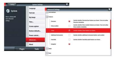
Once CZone is enabled, an additonal CZone menu appears at the bottom of the Settings page.
